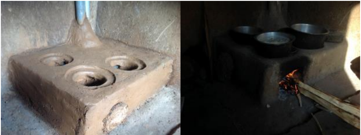
The firewood saving stove that accommodates three cook items at once with one inlet for firewood as opposed to the traditional one with 3 firewood entry spaces and one cook place. This stove saves more than 60% of the firewood that would otherwise be used.
